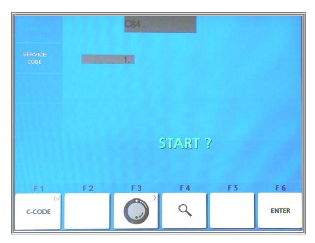
Close the wheel guard and start the extended measurement run by pressing the START KEY.
