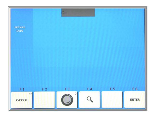
Calibration is completed and must be stored by entering C90.
