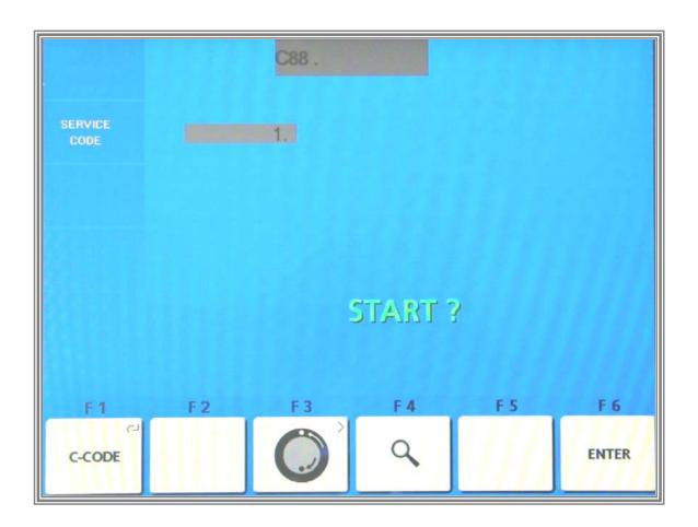
Clamp the test rotor on the main shaft, enter distance, 15" diameter and 6.5" width.
