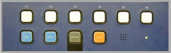
Remove the 100 gm calibration weight from the left-hand plane of the test rotor and insert it into the right-hand plane of the test rotor. Then press the *START KEY*.
