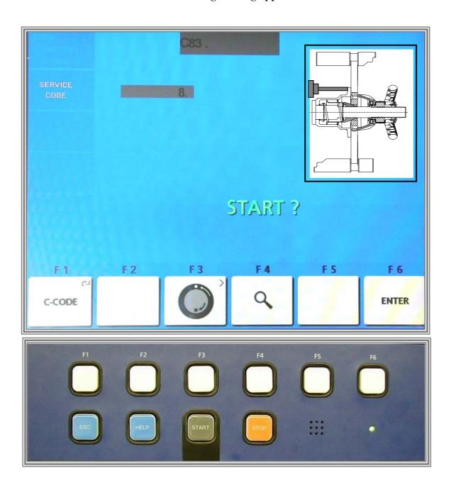
Insert the calibration weight supplied with the machine at the **left inner** side of the adaptor flange. Press the *START KEY*.
