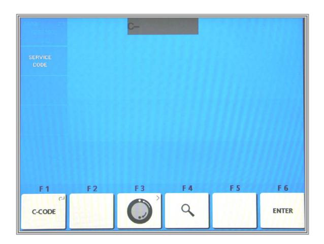
Calibration is completed and must be stored by entering Code C90.
